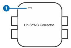
POWER LED: The LED will illuminate in blue when the power is connected.
